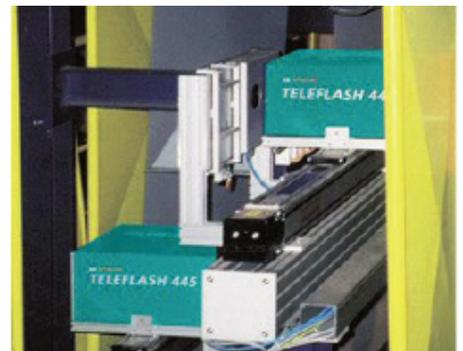
In-line Color and Gloss Measurement with TeleFlash® 445 and GlossFlash 6060 for the Coil Coating Industry
