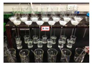
**Fig 3.** Retention of PbSO<sub>4</sub> precipitate using Whatman Grade 40 filter paper.
