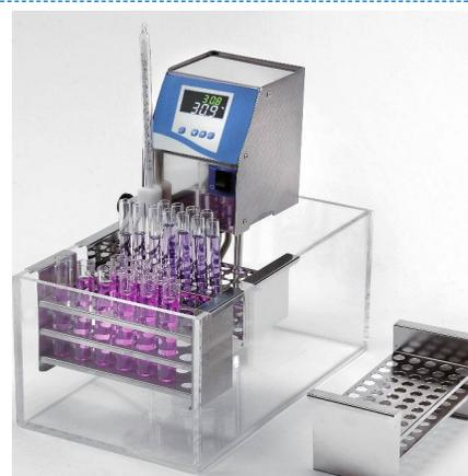
**Metal baths.** Manufactured with a double external AISI 304 stainless steel skin and an AISI 304 stainless steel pressed bath interior.
