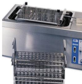
**Racks:** made of AISI 304 stainless steel.
