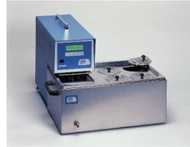
Ring set lid 105, 80, 60 and 37 mm Ø reduction rings and a check thermometer location hole in the lid.
