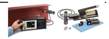
greatly reduces user effort and the risk of influencing the pulling process. Self-aligning aluminum dollies enable accurate measurements on smooth or uneven surfaces
