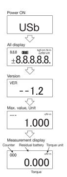
(7) If selected "BATT": Enables auto power off and residual battery indicator functions. If selected "USB": Disables auto power off and residual battery indicator functions.
