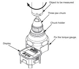
Make sure to hold the chuck holder when rotating the three-jaw chuck.
