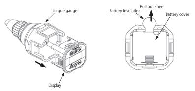
· Turn on the power of the torque gauge and make sure that there is enough battery remaining.
