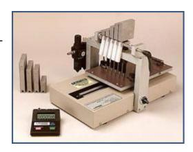
A gantry supports five independent splined-fingers, which provide a constant, vertical load on interchangeable scratch pins (1.0mm or 7.0mm diameter hemisphere). The gantry system includes a handle to raise and lower the arms. In addition, five support rests are incorporated to allow one or more arms to be moved to an upright, rest position such that the arm does not contact the specimen during testing.
