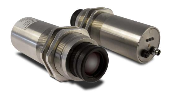
Infrared temperature switch for non-contact detection of hot metal parts or overheating, thereby triggering switching operations which are used for sorting or activating a cooling or similar.
