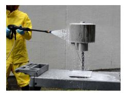
\*As per Keystone Compliance, PA Testing; ENVIRONMENTAL TEST REPORT 1712-067NA-1 REV. N/C, TEST STANDARDS: IEC 60529.
