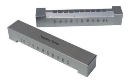
The Sag Tester also known as Anti-Sag Tester, is a simple product used to establish a coatings resistance to sag due to gravity. The Sag Tester is manufactured from corrosion resistant stainless steel, with a total film width application of 75mm equally divided into 10 gaps, incremented in depths of 25µm with distinctive identification for each.
