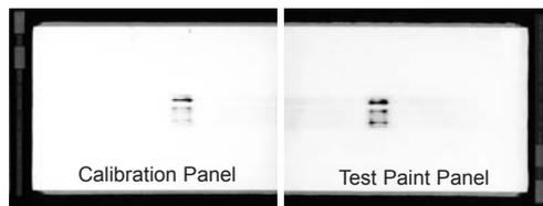
Illustrates simultaneous side-by-side scrubbing of half-panels to maximize correlation, analogous to ASTM D 2486, Method B.
