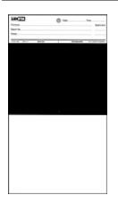
Form N2A-2 is a black and white Unsealed Test Chart. The top is black, and bottom is white with overall dimensions of  $5-1/2 \times 10$  in (140 x254) mm).
