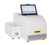
humidity and flow rate precisely, guaranteeing the testing sensitivity and repeatability of test results. C330H is applicable to determination of water vapor permeability of plastic films, sheeting, paper, packages and other relative packaging materials in food, pharmaceutical, medical apparatus, consumer goods, photovoltaic and electronic industries, etc.
