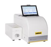
rate precisely, guaranteeing the testing sensitivity and repeatability of test results. C330G is applicable to determination of water vapor permeability of plastic films, sheeting, paper, packages and other relative packaging materials in food, pharmaceutical, medical apparatus, consumer goods, photovoltaic and electronic industries, etc.
