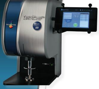
The Technidyne TEST/Plus<sup>™</sup> ISO Brightness combines industry standardized measurement technology with an innovative control package that allows the user to tailor build their testing and evaluation capabilities. This new addition to the TEST/Plus<sup>™</sup> product line is built to meet your ISO Brightness testing needs;
