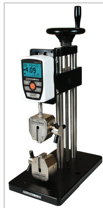
Shown with an ES20 test stand and G1061 wedge grips
