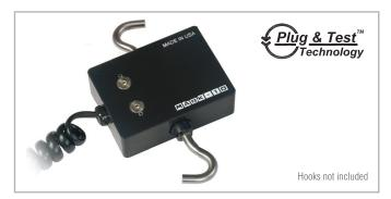
Series R03 smart sensors are designed for tension and compression measurement applications in virtually every industry. Threaded holes on two sides can accept a variety of hooks and implements, making this sensor particularly well suited for inline tests. Capacities available from 0.25 to 100 lbF [1 to 500 N]. Compatible with Mark-10 indicators (sold separately) through unique Plug & Test™ technology.
