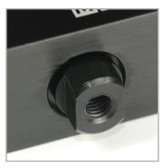
^ The load cell shaft includes flat surfaces as well as a threaded hole to accommodate attachments.
