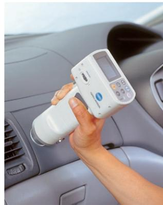
The measuring head can be used independently of the data processor. This is advantageous when portability is required or limited space is available.
