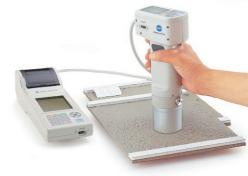
The compact data processor features a built-in printer for superior mobility.
