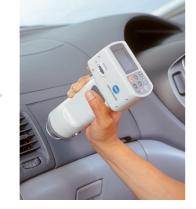
The measuring head can be used independently of the data processor. This is advantageous when portability is required or limited space is available.
