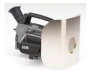
The new GF309 is equipped with a special midwave "flame filter" for high temperature (up to 1500°C) furnace inspections and boiler inspections. Additionally, the nickel coated heat shield contoured to improve worker safety and comfort during inspection.
