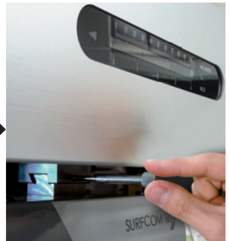
The detector is locked and unlocked by a half turn clockwise or counterclockwise respectively.
