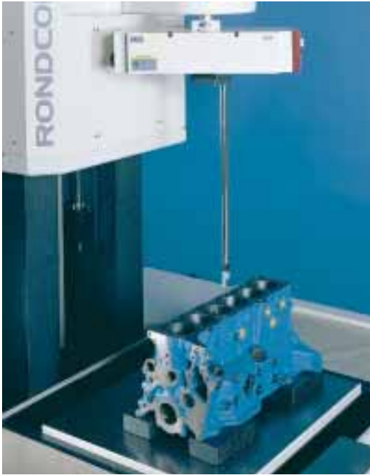
Examples of typical applications for Rondcom 72/75: measurement of cylinder heads, engine blocks and crankshafts
