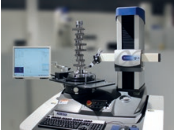
An example of measuring a crankshaft using an exclusive jig tool
