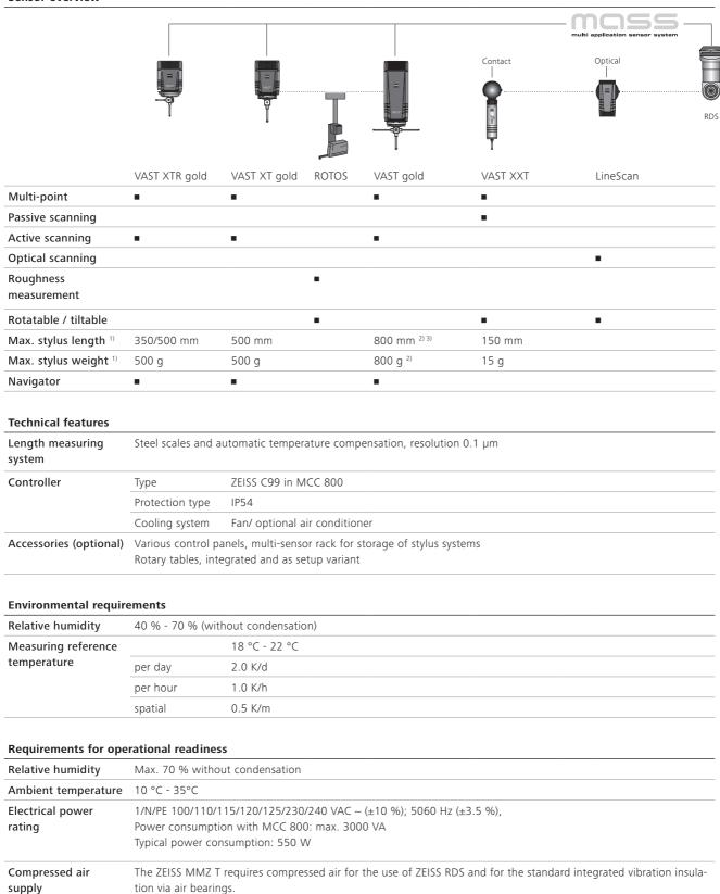
Supply pressure 6-10 bar (87-145 psi), pre-cleaned. Air quality complies with ISO 8573 part 1: Class 4
