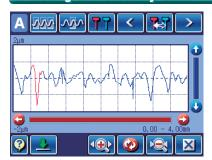
With the Surftest SJ-310, you can delete portions of measurement data. This feature allows you to make new calculations by deleting data that should not be included in parameter calculation, such as data on a scratch.
