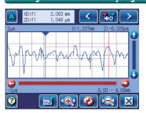
You can not only magnify or shrink waveforms, but also calculate the coordinate difference between two points using a ruler operation.
